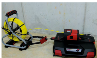
RM35 with belt and clip system connected to GF4.5 fiberglass rod
